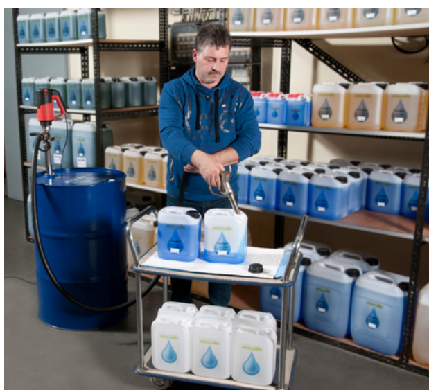
The pump FP 425 S in operation for conveying a particularly high-quality lubricant.
