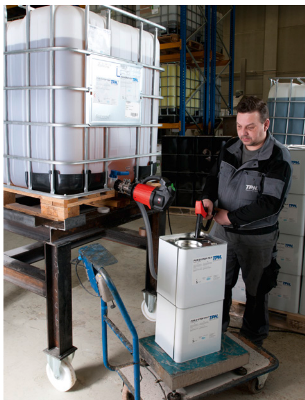
Fast container filling from the IBC outlet.
