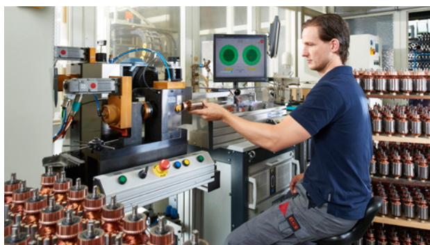
Anchor test in the winding department.
