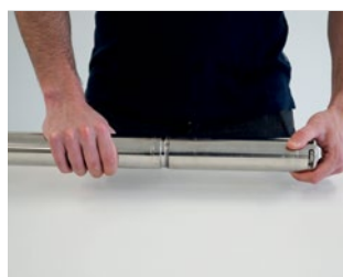
Unscrew stator housing
