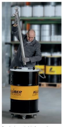
Required room height for erection: Approx. 2200 mm, without motor
