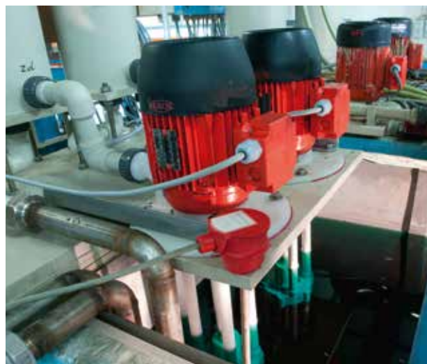
F 716 – circulating chemicals in a pickling tank.
