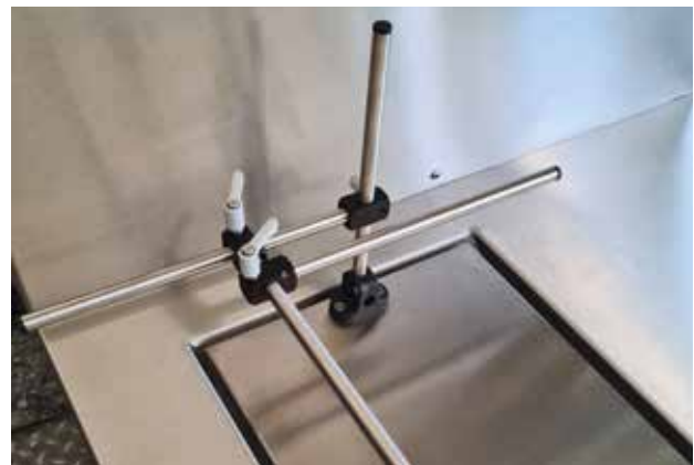
Toolless adjustment of the limit stop.
