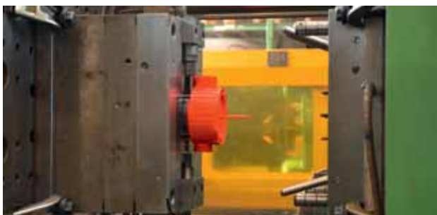
Own injection moulding production, here for the housing of an FMC.
