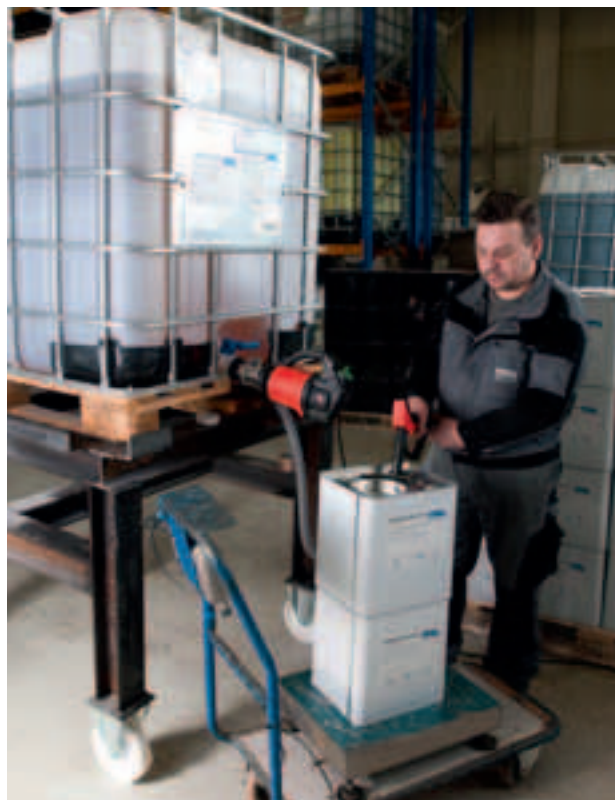
Fast container filling from the IBC outlet.
