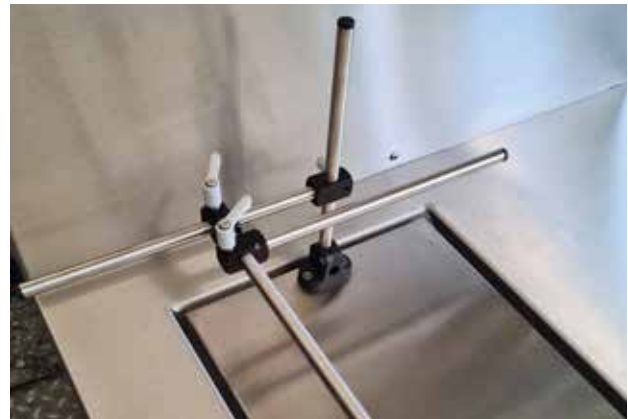
Toolless adjustment of the limit stop.
